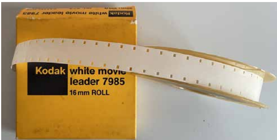
Figure 3. A roll of Kodak 16 mm film leader that was used to construct “tapes” that arranged reinforcers according to variable-interval or variable-ratio schedules.
