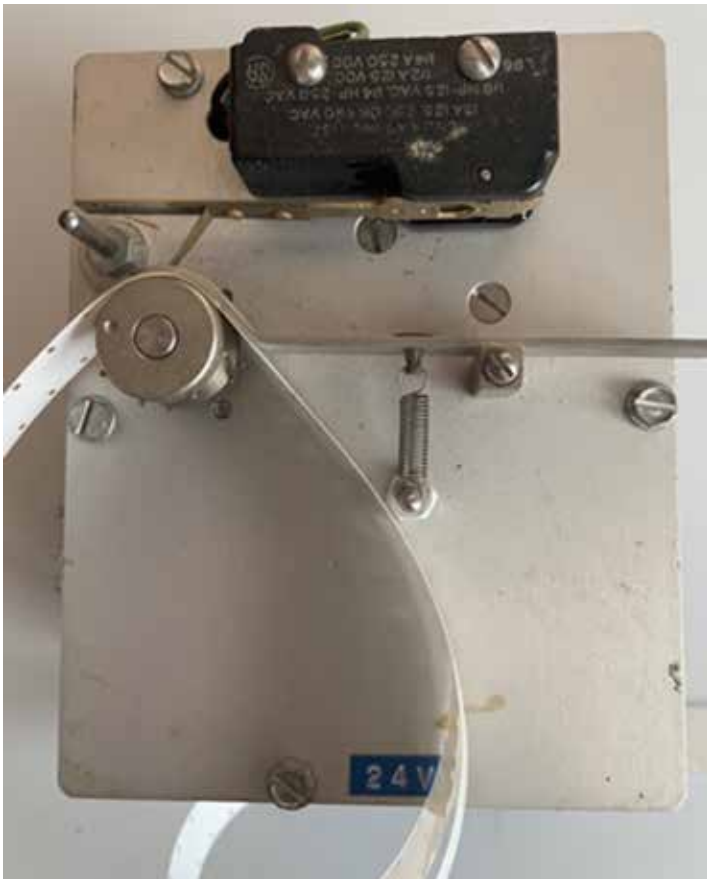
Figure 2. A device for programming a variable-interval or variable-ratio schedule. See text for construction and operation details.
