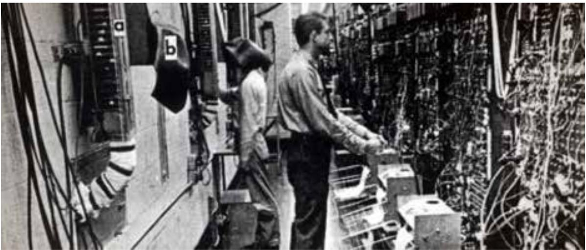
Figure 2. Ogden Lindsley in the first human operant lab, located at Waltham State Hospital in Massachusetts. The figure of interest is the “headless horseman” behind Lindsley and to his left. The labels “a” and “b” are on, respectively, a reinforcer dispenser and the head cover for a second behavior scope, not being used.
