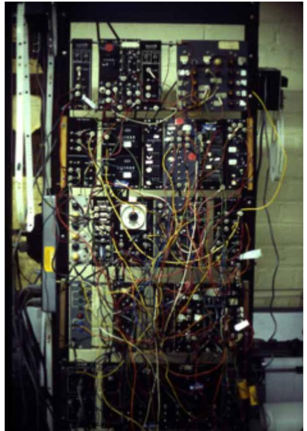
Figure 4. A relay rack with programming modules connected to one another by snap leads (the colored wires) to create a program controlling an operant conditioning experiment.
