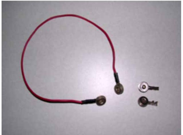
Figure 2. In the lower right, a pair of snap connectors, labeled Nu-Way. These connectors could be soldered to a length of wire to create the snap lead shown in the center of the photograph.
