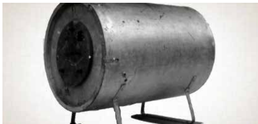
Figure 4. A "candy barrel" operant conditioning chamber of the sort reported by Heron and Skinner (1939). The rat work area is located behind the dark circle in the center of the left end of the barrel. It pulls out, revealing a 6 inch or so diameter tubular-shaped chamber with a hole in the top for inserting the rat.
