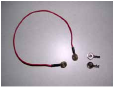
Figure 2. In the lower right, a pair of snap connectors, labeled Nu-Way. These connectors could be soldered to a length of wire to create the snap lead shown in the center of the photograph.
